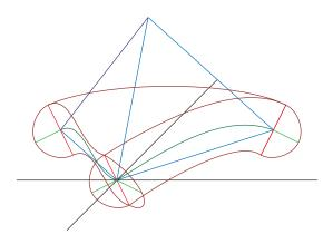
To build the scaffold for the offset surface and the offset of the delimiting curve and points for simplicity will focus on the original a-patch interpolating three points on the tetrahedron. The most natural scaffold is a prismatic scaffold, then one may add a baricentric point in each prism to divide it in 6 tetrahedrons.
