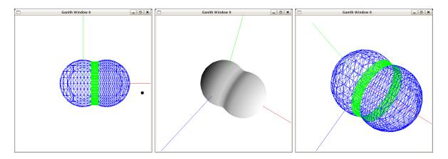
Figure 4: Inner offset of two spheres, clipped at the intersection planes
