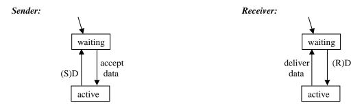
Figure 40.3 Sender and receiver models for the simple protocol
