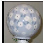
Spherical microphone array
