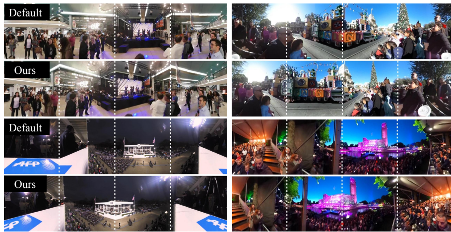
Fig. 7. Qualitative examples of default CANONICAL cubemaps and our snap angle cubemaps. We show failure cases here. In the top left, pixel objectness [3] does not recognize the stage as foreground, and therefore our method splits the stage onto two different cube faces, creating a distorted stage. In the top right, our method creates a distorted train by splitting the train onto three different cube faces because pixel objectness does not recognize the train as foreground.
