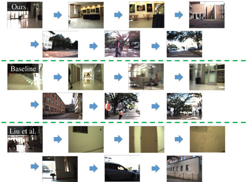
Fig. 4.18 Example keyframe selections for the robot video. Top result is produced by our snap point method, middle result is the event segmentation baseline, and bottom result is the existing method of [32]. We see that our snap point-based method was able to pick a representative frame for each location that the robot visited. The other two summaries contain blurry or uninformative frames
