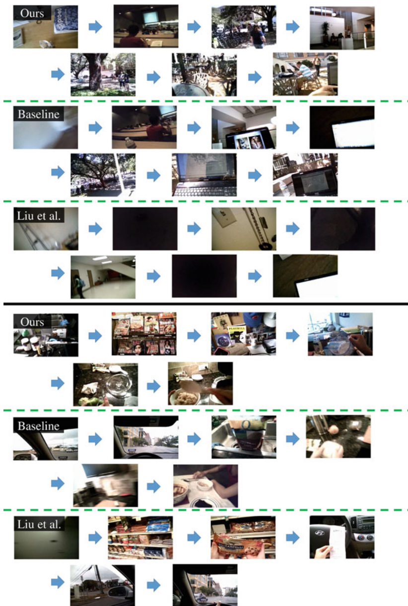
Fig. 4.17 Example keyframe selections for two 4-h ego videos. Top result is produced by our snap point method, middle result is the event segmentation baseline, and bottom result is the existing method of [32]. While our method generally appears to outperform the baselines, it can make mistakes as well. Our method picks a frame of a bunch of books on a bookshelf in the second event of the second video (see the second frame in the seventh row ), when it would be preferable to pick a frame of groceries as done by the method of [32] (see the second frame in the second last row ) since the main event was groceries shopping
