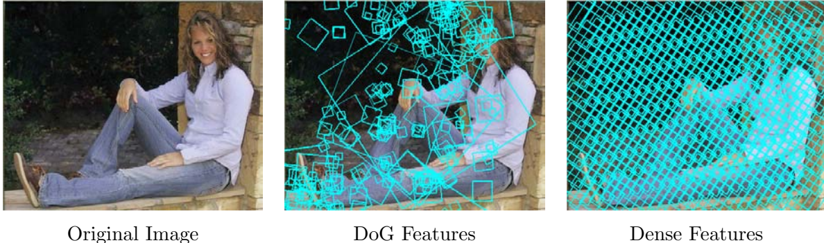
Figure 3.2: DoG vs. Dense Features - An example of the difference between the points selected on an image (left) by difference-of-Gaussians or DoG (middle) and dense feature selection (right). We use dense feature selection on our Hot or Not data to ensure that a significant number of features are selected from all parts of the person in the image.
