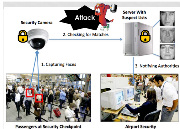
Figure 1. We present an attack on a secure face identification system using both cryptographic and computer vision tools. While the system ought to maintain the privacy of both the suspect list and passengers, our attack recovers coded versions of their faces and sketches human-understandable images from those codes.
