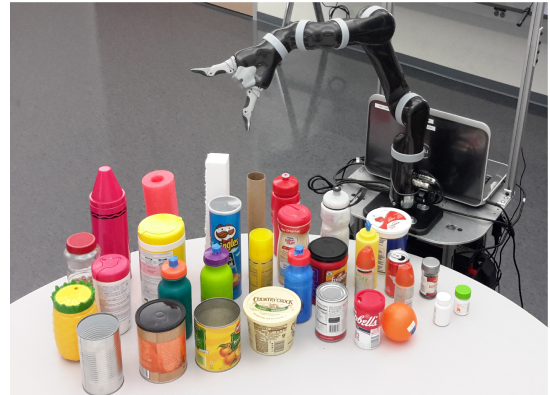
Figure 1: The robot used in our experiments, shown here with the 32 objects it explored in order to learn three ordinal properties: weight , width , and height .
