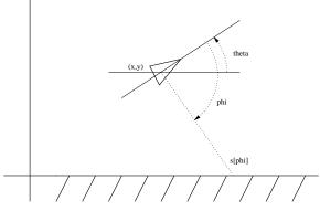
The robot is at position (x, y) and orientation  $\theta$ . The range sensor in direction  $\phi$  senses distance  $s_{\phi}$ , but in this paper we assume that y and  $\theta$  are sensed directly.
