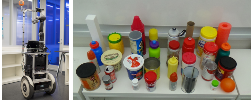
Fig. 2: The robot used in our experiment, and the objects explored by the robot for grounding perceptual predicates.
