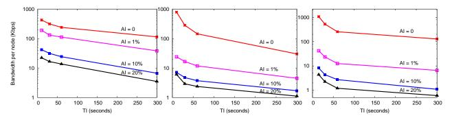
Figure 8: Load vs. AI and TI for (a) DHH, (b) PrMon, and (c) DDoS detection. AI and TI significantly reduce the monitoring load for the three applications; y-axis is on a log scale.
