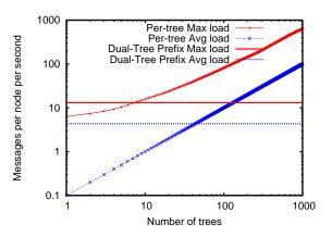
Figure 14: Break-even point for NI tracking overhead as the number of trees (attributes) varies for (a) pertree aggregation vs. (b) dual-tree prefix aggregation in a 1000-node system. The break-even points for the average and maximum load are 44 trees and 8 trees.
