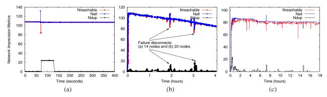
Figure 9: NI metrics under system churn: (a) single node failure at 70 seconds for 108 Emulab nodes, (b) periodic failures for 108 Emulab nodes, and (c) 85 PlanetLab nodes with no synthetic failures.
