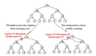
Figure 2: Dynamically-constructed aggregation hierarchies raise two challenges for guaranteeing the accuracy of reported results: the *failure amplification effect* and *double counting* caused by reconfiguration.
