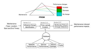
Figure 1: PRISM Overview and design.
