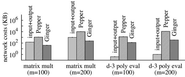
Figure 6—Per-instance network costs of GINGER and its base (PEPPER [48]), compared to the size of the inputs and outputs. At this batch size ( $\beta = 5000$ ), GINGER’s refinements reduce per-instance network costs by a factor of 20–30 compared to PEPPER. GINGER’s network costs here are hundreds of KB or less. The y-axis is log-scaled.
