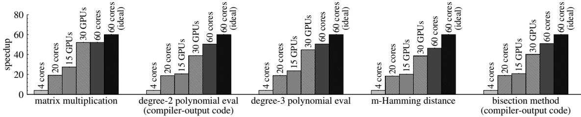
Figure 10—Latency speedup observed by GINGER’s verifier when the prover is parallelized. We run with  $m = 100, \beta = 120$  for matrix multiplication;  $m = 256, \beta = 1200$  for degree-2 polynomial evaluation;  $m = 100, \beta = 180$  for degree-3 polynomial evaluation and  $m$ -Hamming distance; and  $m = 25, \beta = 180$  for bisection method. GINGER’s prover achieves near-linear speedups.
