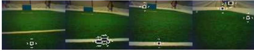
Fig. 8. Some typical errors on a field with no motion. The overlaid squares only indicate discontinuities, and enough of these squares must appear in the same sector for motion to be detected there. In the run from which these images were taken, in which there was no motion on the field, 83% of the frames contained no discontinuities of this type, and over 95% of the image sectors were correctly labeled as containing no motion.
