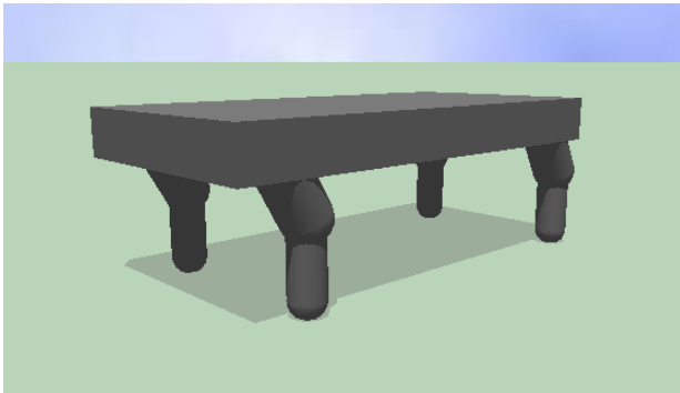
Fig. 14: The quadruped robot model with knees. This model extends the quadruped in Fig. 6 by adding knee joints. The hip joints allow the legs to swing forward and backward up to 30^\circ in each direction. The knee joints allow the lower part of the legs to swing only forward (up to 30^\circ ) with respect to the upper part. This model provides a more challenging platform to evaluate how well ENSO scales up to larger problems with more modules.
