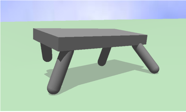
Fig. 6: The quadruped robot model. The legs are attached to the body by hinge joints with axes of rotation tilted sideways, allowing the legs to make full circular rotation. Locomotion is achieved by coordinating the circular movements of the legs. Although more legs and complex legs can be used, this model is a simple and physically realistic platform that has symmetric and modular controllers, and is therefore suitable for evaluating ENSO on challenging environments.
