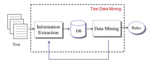
Figure 1: Overview of IE-based text mining framework
