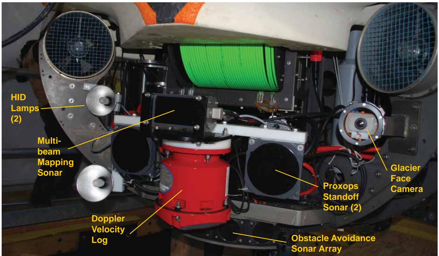
**Figure 9:** Glacier mapping and imaging array
