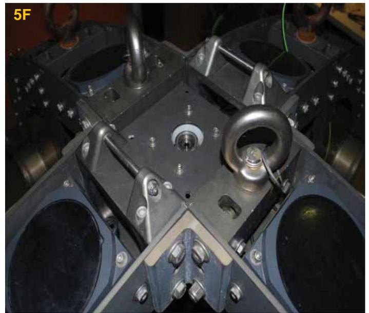
Figure 5: Final Stage Return-to-Melthole Navigation: 5A through 5E) machine vision frame captures of the auto location and return system in action on Mission 5; 5F) the zenith-pointing machine vision camera.
