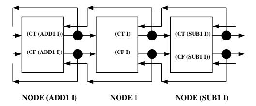
Each node behaves in the following way: A bit is encoded by double-rail coding. **TRUE** is represented by the C-element **CT** being **TRUE**, and the other C-element **CF** being **FALSE**. **FALSE** is represented by the opposite configuration. If the node is empty, both C-elements are **FALSE**; never will both C-elements be **TRUE** simultaneously. This is because this circuit requires (and maintains) that if two adjacent nodes are non-empty, they must also represent the same value.
