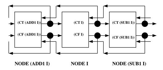
Each node behaves in the following way: A bit is encoded by double-rail coding. **TRUE** is represented by the C-element **CT** being **TRUE**, and the other C-element **CF** being **FALSE**. **FALSE** is represented by the opposite configuration. If the node is empty, both C-elements are **FALSE**; never will both C-elements be **TRUE** simultaneously. This is because this circuit requires (and maintains) that if two adjacent nodes are non-empty, they must also represent the same value.
