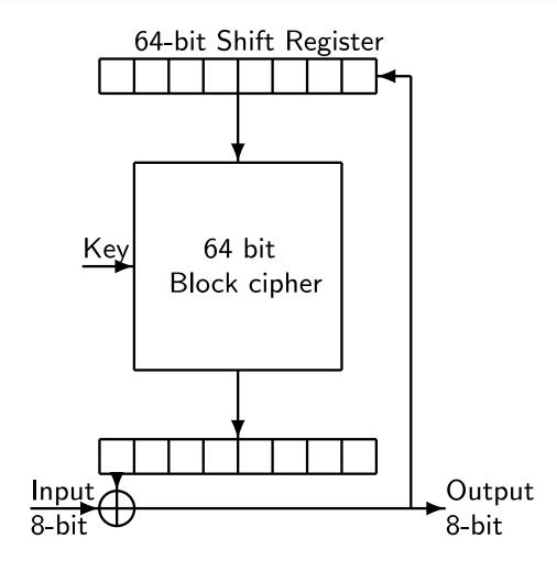
In Cipher Feedback mode (CFB) each input byte is XORed with the first block of the previous output and fed back into the encryption.
