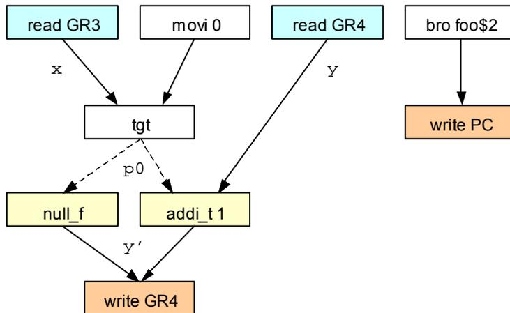
Based upon the predicate, variable  $y$  is either incremented or left unchanged. A similar approach may be used to nullify stores. In that case, the target of the NULL instruction is a store instruction instead of a write instruction.
