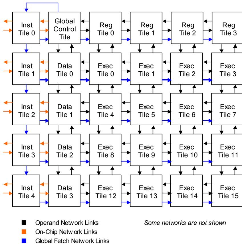
This approach (referred to as a Grid Processor Architecture) fits well with future semiconductor technologies. It allows faster clock rates than conventional approaches, while also providing superior instruction-level parallelism and extensibility.
