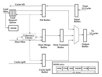
Fig. 6. Block diagram of the MHU. Inset shows the logical structure of the MSHRs
