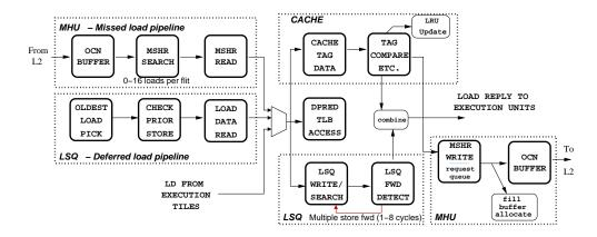
Fig. 2. The DT Load Pipelines
