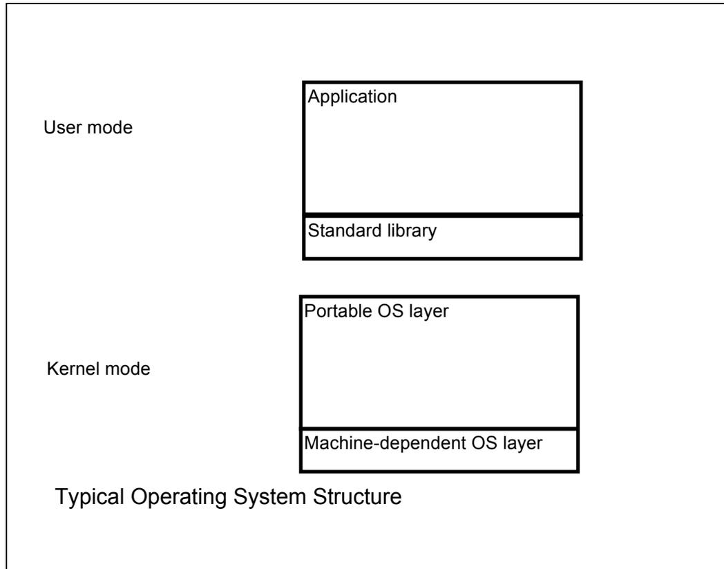
Also, want OS to be portable, so put a layer that abstracts out differences between different hardware architectures (e.g. Linux runs on x86 and ARM, Solaris runs on SPARC and x86, NT/win2k runs on x86 and (until recently) Alpha)
