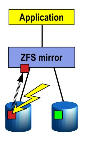
**<u>2.</u>** ZFS tries the second disk. Checksum indicates that the block is good. **<u>3.</u>** ZFS returns good data to the application and repairs the damaged block.
