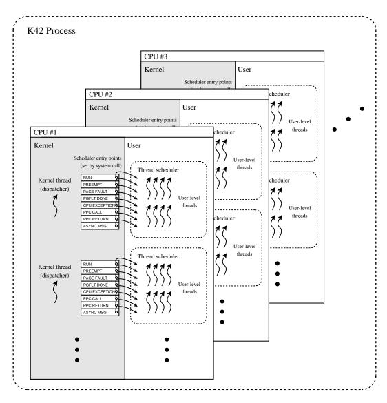
Figure 3.1: Diagram of a single process in K42.
