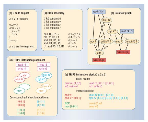
consuming instructions mapped on the execution array. The compiler converts the original branch to a test instruction and uses the result to predicate the control-dependent instructions, shown as dotted lines. By converting branches to predicates, the compiler creates larger regions with no control flow changes for more effective spatial scheduling.
