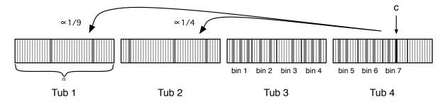
Figure 6: Illustration of the tub protocol from peer c's perspective. Shaded entries represent peers that c can contact for a trade when appropriate. Note that c only uses bins for its own tub and the immediately preceding one.
