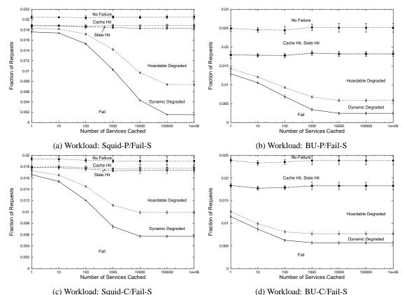
Figure 8: Service failure rate v. number of cached service extensions (*simulation results.*)
