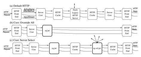
Figure 1: Example service/extension program pipeline of (a) standard HTTP protocol, (b) completely overridden protocol, (c) partiallyoverridden protocol.
