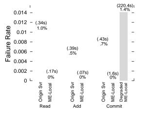
Figure 9: Failure rate and response time for catalog application.
