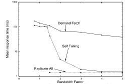
Fig. 7: Read response time as available bandwidth varies for full replication, demand reads, and self-tuning replication.
