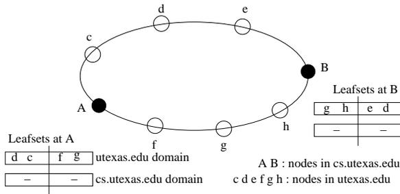
Figure 5: Concurrent joins leading to path convergence property violations. Nodes A and B in `cs.utexas.edu` join concurrently using nodes in `utexas.edu` domain as bootstrap nodes. Observe the incorrect leafset tables at node A and B corresponding to `cs.utexas.edu` domain.
