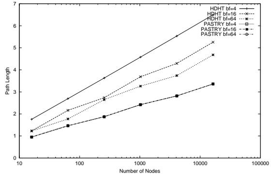
Figure 7: Average path length to root in Pastry versus ADHT for different branching factors. All Pastry lines overlap as the branching factor does not effect the Pastry routing procedure.
