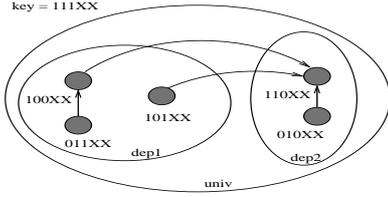
Figure 1: Administrative autonomy violation in a bit-correcting DHT.
