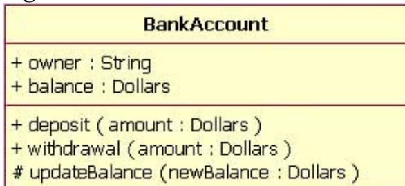
Figure 15: A BankAccount class that shows the visibility of its attributes and operations
