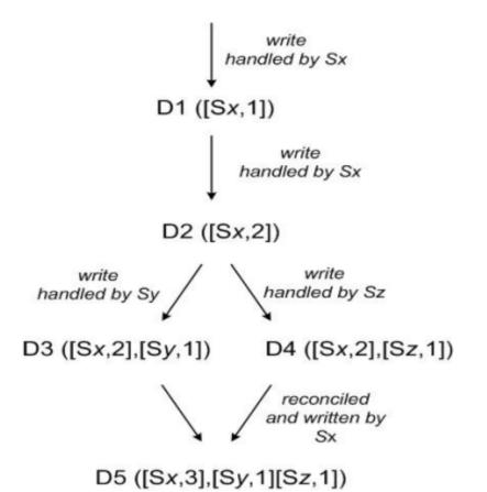
Figure 3: Version evolution of an object over time.
