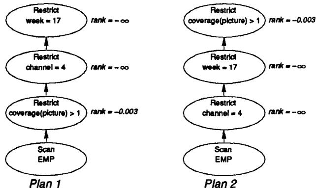
Figure 1: Two Execution Plans for Example 1
