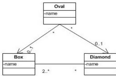
constraint: oval is connected to Box or Diamond, but not both
