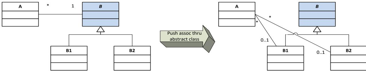
By making class A associations reference abstract class B’s subclasses, a constraint must be added: each A instance is bound to a B1 or B2 instance, but never both.
