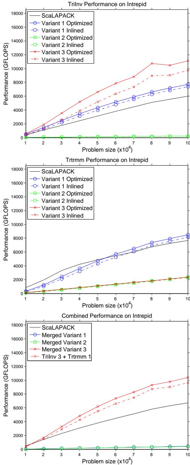
Figure 5: Performance results comparing algorithmic variants and ScaLAPACK on Intrepid. 2/3 of theoretical peak is at the top of the graphs. Variants 2 and 3 of TRTRMM are almost the same, so they appear on top of each other in the graph. Variant 3 is slightly faster.
