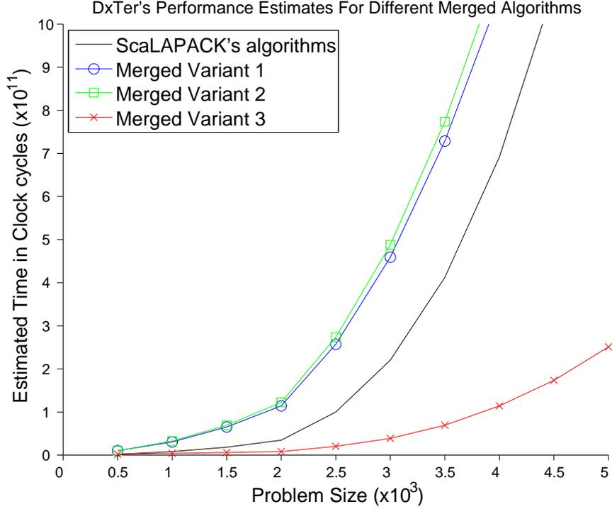
Figure 2: Performance Estimate of different merged algorithms compared to ScaLAPACK's unmerged algorithms
