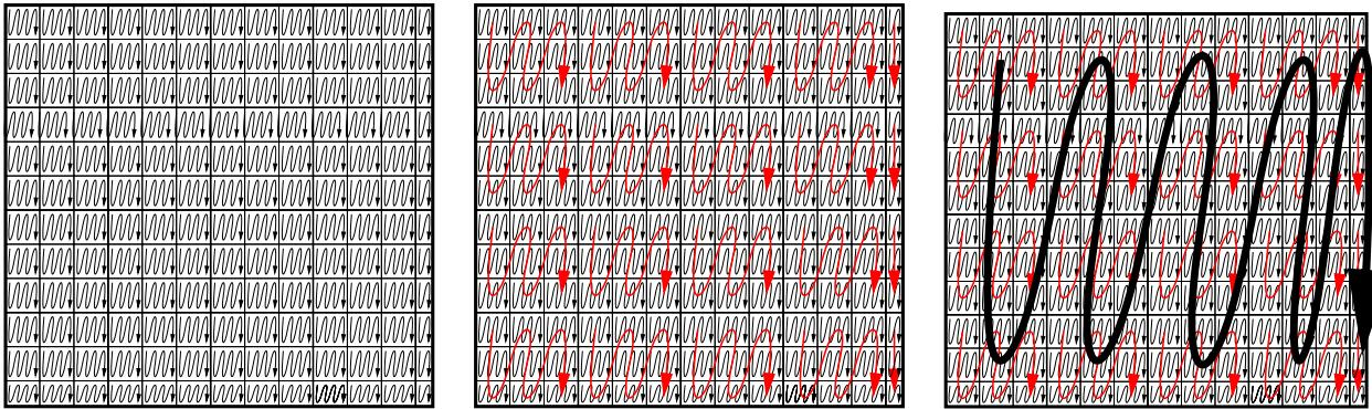
Figure 3: Generalized Morton order: The lowest level blocks are  $5 \times 5$  matrices stored in column-major order. The next level consists of  $3 \times 3$  blocked matrices, stored in column-major order. Finally, those blocks are stored in column-major order themselves. Notice that the traditional Morton order can be achieved by picking the blocking at each level to be  $2 \times 2$  for  $\log_2(n)$  levels, storing each level in row-major order.
