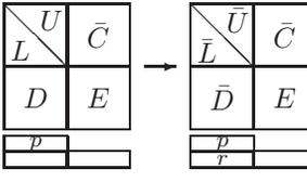
Here,  $\bar{U}$  overwrites the upper triangular part of  $B$  (where  $U$  was stored before this operation). The lower triangular matrix  $\bar{L}$  that results needs to be stored separately since both  $L$ , computed in Step 1 and used at Step 2, and  $\bar{L}$  are needed during the forward substitution stage when solving a linear system.
