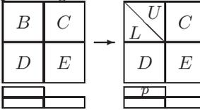
**Step 2: Update  $C$**  consistent with the factorization of  $B$  (using forward substitution):
