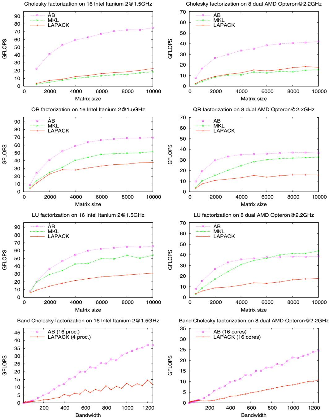
Figure 10: Performance of the multithreaded factorization algorithms.
