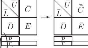
Again, care must be taken in this step to exploit the zeroes below the diagonal of the upper triangular matrix produced in the previous step. This structure-aware procedure, though not equivalent to a clean triangular system solve (plus the application of the corresponding permutations), can be performed in terms of level-3 BLAS and presents essentially the same computational cost, modulo a lower order term. For details, see algorithm  $\text{FS}_{\text{BLK}}^{\text{SA-LIN}}$  in [30].
