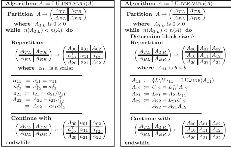
Figure 1: Unblocked and blocked algorithms (left and right, respectively) for computing the LU factorization (without pivoting). Here,  $n(B)$  stands for the number of columns of  $B$ .
