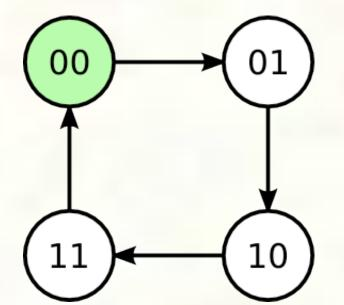
Counter starts at 0 (green) and increments each time the clock cycles, until it gets to 3 and then overflows back to 0.
