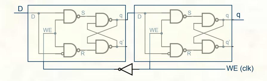
Note: a **flip-flop** is an **edge-triggered** storage element. Edge-triggered means the stored data can be changed when the clock changes voltage, either from low to high (as here) or high to low.
