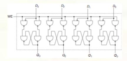
■ A 4-bit register using D latches
