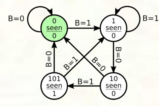
B is input signal to the lock, X is output signal to unlock
