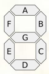
2-bit counter will need to display digits 0-3, so will output a 1 for each segment to be lit for a given state
