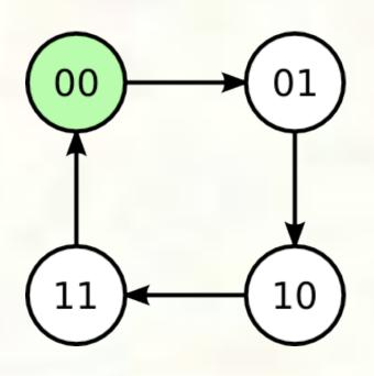
Counter starts at 0 (green) and increments each time the clock cycles, until it gets to 3 and then overflows back to 0.
