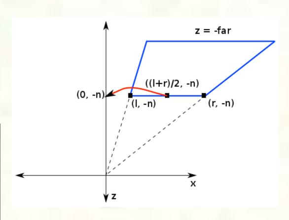
Step 1: Shear to center on –z axis
