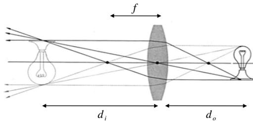
For a “thin” lens, we can approximately calculate where an object point will be in focus using the the Gaussian lens formula:
