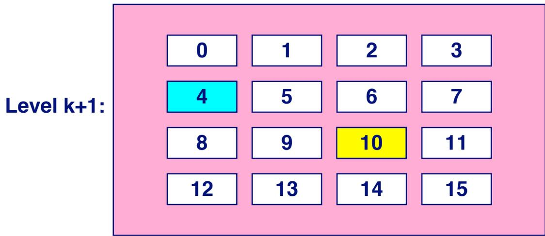
Larger, slower, cheaper storage device at level k+1 is partitioned into blocks.
