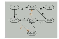
**Definition**  $\Gamma(\mathcal{N})$ : Vertices are wires of  $\mathcal{N}$ ; directed edges drawn for non-sequential wire pairs.
