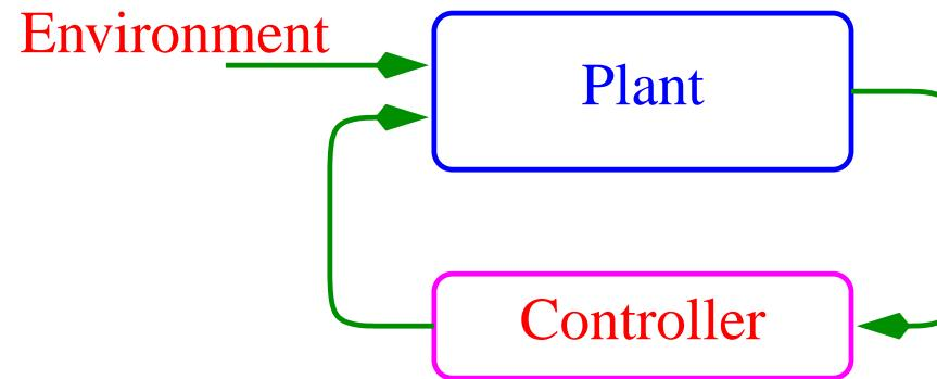
Required: A design for a **controller** which will cause the **plant** to behave correctly under all possible (appropriately constrained) **environments**.
