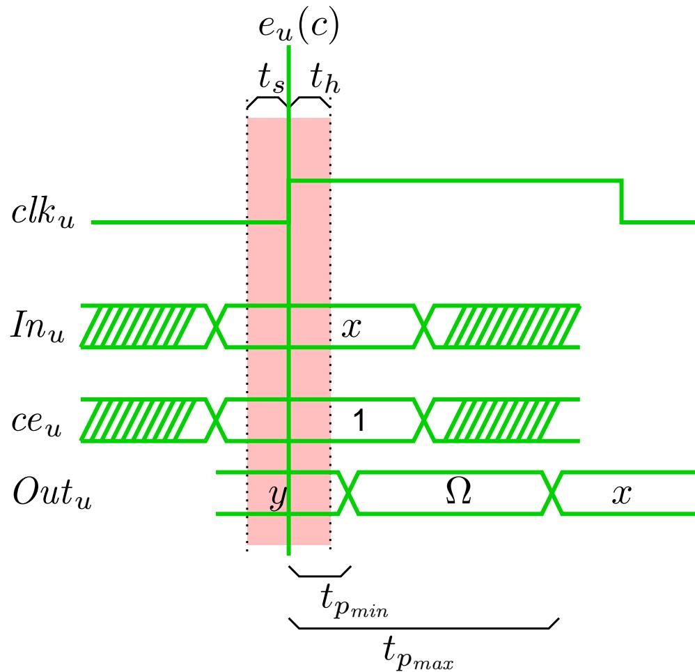
Transition after  $t_{p_{min}}$ . Final value after  $t_{p_{max}}$
