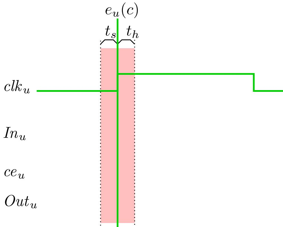
Setup and holding times determine a “metastability window”.
