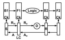
Fig. 1. A Pipeline Stage with A Latch Controller Network.
