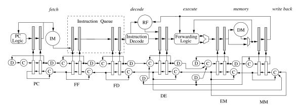
Fig. 4. High-Level Organization of Desynchronized 6-Stage Pipelined Processor Model
