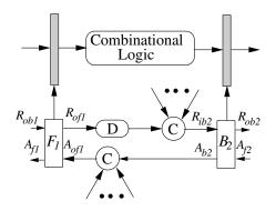
Fig. 3. DFVD Controller Circuit for Data Transfer
