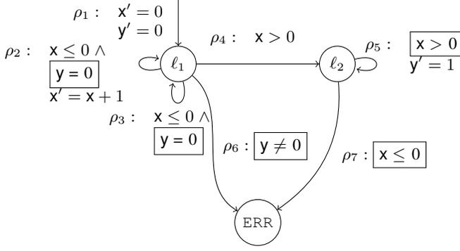
Fig. 3: The transformation of the program from Figure 1 for the sub-property  $\text{AGEF } y = 1$  to be utilized in the verification algorithm. The nested property  $\text{EF } y = 1$  is substituted with its precondition resulting in a transformation for  $\text{AG } ((\text{pc} = l_1 \Rightarrow y = 0) \vee (\text{pc} = l_2 \Rightarrow x > 0))$  instead.
