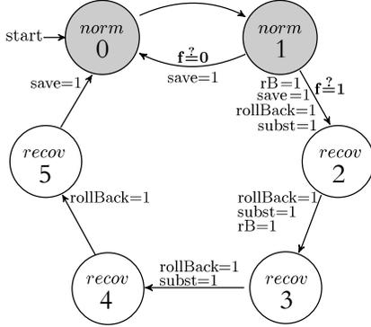
Fig. 6: FSM of the DTR control block: “ $\overset{?}{=}$ ” denotes a guard, “ $=$ ” an assignment and, by default, signals are set to 0.
