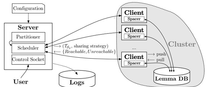
**Figure 1.** SMTSERVICE framework overview. The server implements Algorithm 1. Each client represents a different solver process in a computing node. Solid lines represent TCP/IP connections, while dashed lines represent disk I/O.
