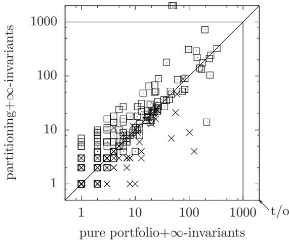
Figure 3. Comparison between sharing invariant with and without partitioning over *less500* sat ( $\times$ ) and *unsat* ( $\square$ ) instances. Compared to “best”, this combination is overall 14% slower while using 75% less CPU. Moreover it is shown that partitioning outperforms on all sat instances.
